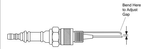
Figure 10 - Spark Plug Gap
